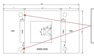
The vessel's bottom deck was divided into 3 watertight spaces, the stern void space with the two hatches open, the middle engine room space with the hatch open, and the remaining forward void space that remained intact and caused the bow to bob along the channel floor.
