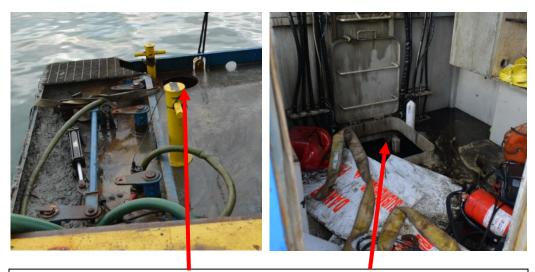
Both stern hatches (port stern hatch pictured) which open to the same compartment were found open. The right picture depicts the engine room hatch open which would have accelerated the downward flooding.
